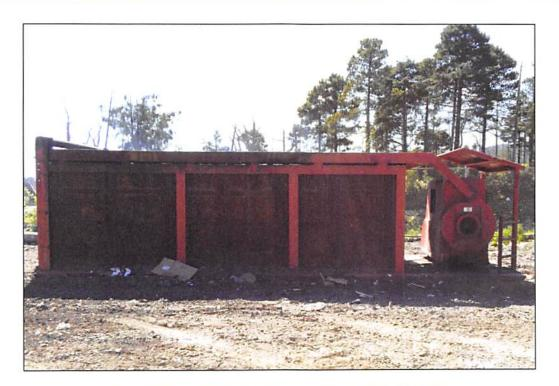
Figure 3-10 Air Curtain Burner at Denny Island Landfill
