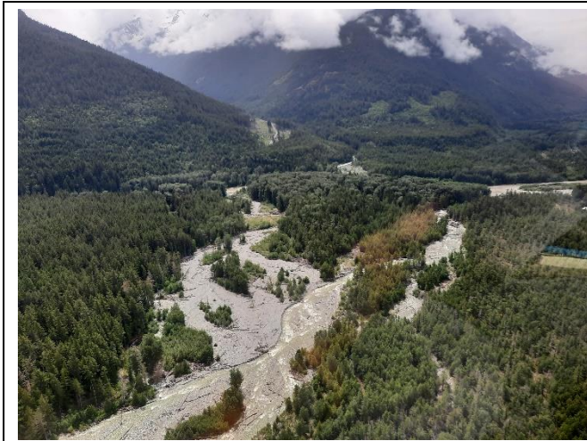
Photo12: Downstream view of Burnt Bridge Creek from above berm area showing water flowing down mainstem and preferred avulsion channel.
