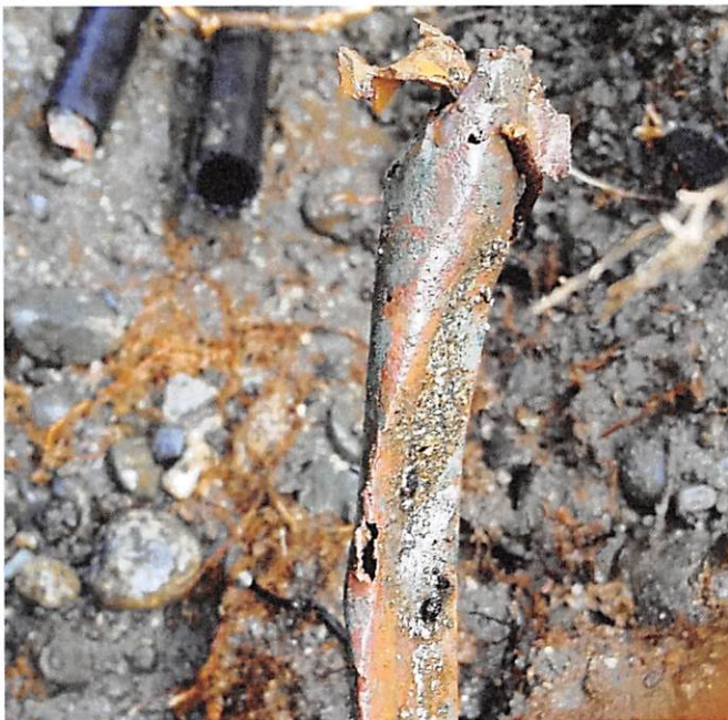
Photo: Rotted out copper service line excavated April 8 th .
