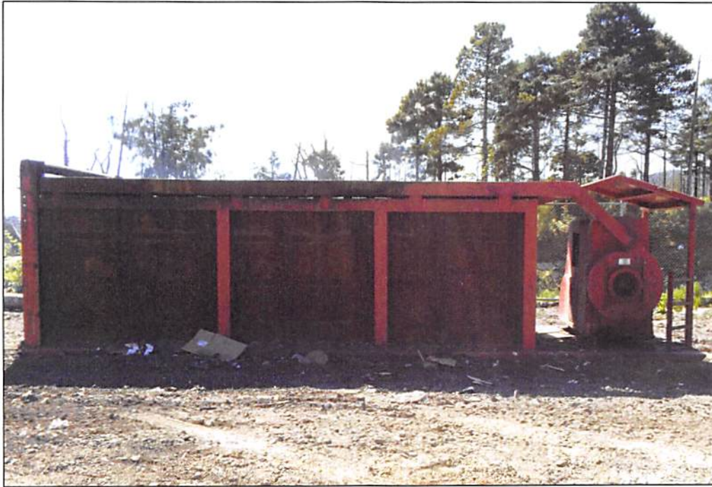
Figure 3-10 Air Curtain Burner at Denny Island Landfill
